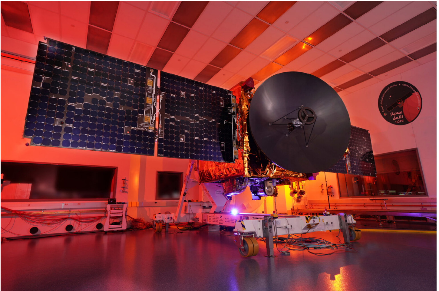
The Emirates Mars Mission Hope Spacecraft prior to shipment to Dubai and the Tanegashima Launch site, with fully deployed solar panels and instruments visible (facing the floor) measuring nearly 5 meters across - Source: LASP News
